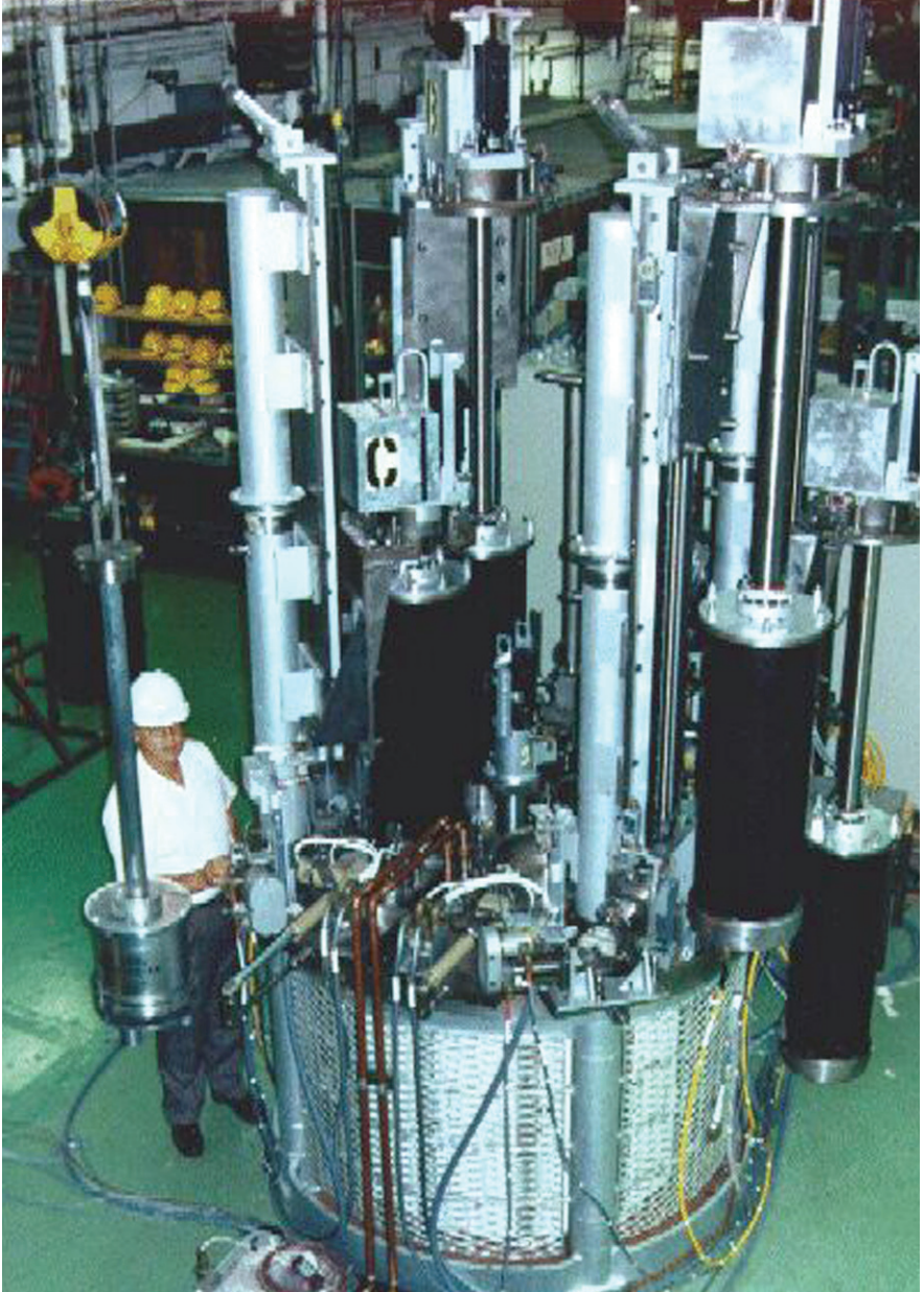
Figure 3: Pilot "Electrorefiner" for Experimental Breeder Reactor II at Idaho National Laboratory. Reprocessing for the TWR would presumably use a similar reprocessing technology. (Source: Wikimedia Commons, author: Argonne National Laboratory, at http://commons.wikimedia.org/wiki/File:EBRElectrorefiner.jpg )
